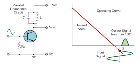
Due to its heavy audio distortion, class C amplifiers are commonly used in high frequency sine wave oscillators and certain types of radio frequency amplifiers, where the pulses of current produced at the amplifiers output can be converted to complete sine waves of a particular frequency by the use of LC resonant circuits in its collector circuit.
