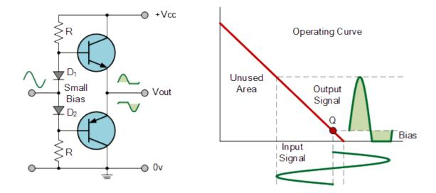
The advantage of this small bias voltage, provided by series diodes or resistors, is that the crossover distortion created by the class B amplifier characteristics is overcome, without the inefficiencies of the class A amplifier design. So the class AB amplifier is a good compromise between class A and class B in terms of efficiency and linearity, with conversion efficiencies reaching about 50% to 60%.
